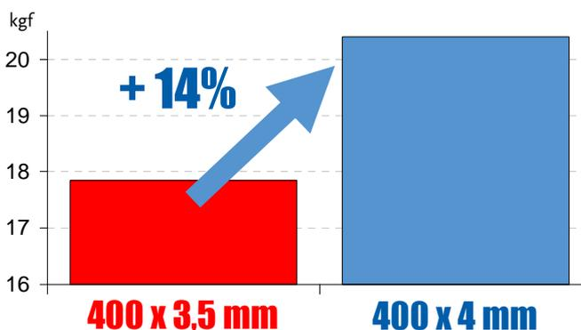
(Values in kgf extended from Standard flexible PVC tearing resistance: 50 N/mm - DIN 53 515 - 1kgf = 1 kilogramme force = 9,8 Newtons)
